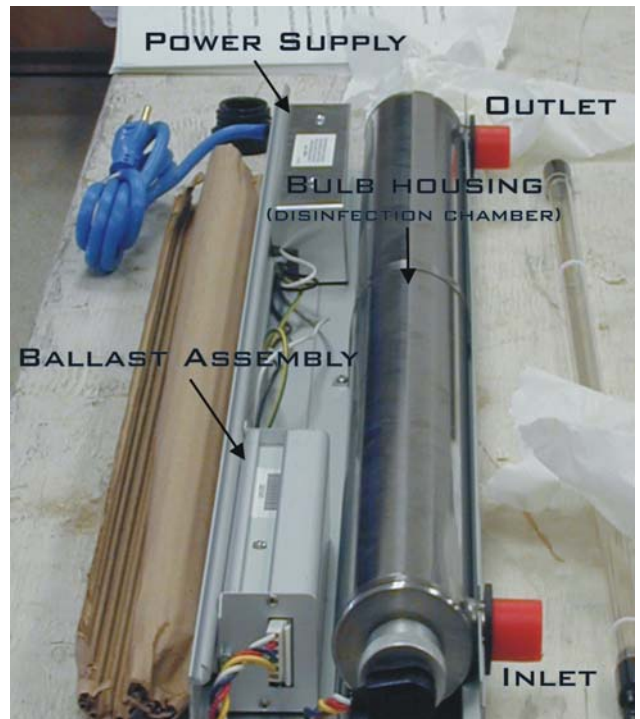
Figure 3: Schematic of UV Unit with Cover Removed
