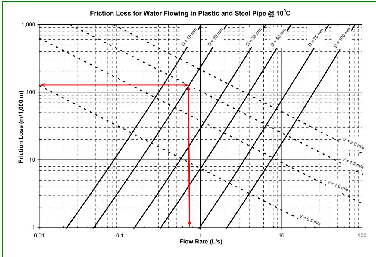
*Graphic Text to Translate: Friction Loss for Water Flowing in Plastic and Steel Pipe @ 10 degrees Celcius; Friction Loss (m/1,000m); Flow Rate (L/s); D =19mm; V=0.5m/s*
