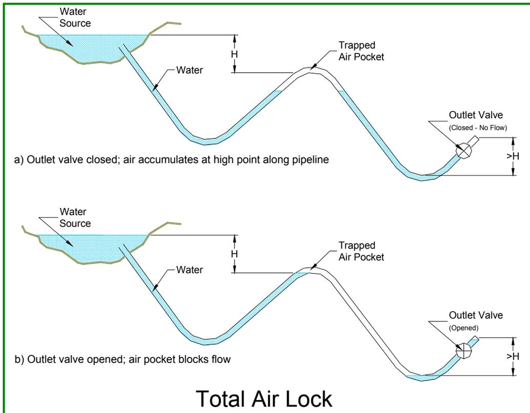
*Graphic Text to Translate: Total Air Lock; Water Source; Water; Trapped Air Pocket; Outlet Valve (Closed – No Flow); a) Outlet valve closed; air accumulates at high point along pipeline; b) Outlet valve opened; air pocket blocks flow; Outlet Valve (opened)*
