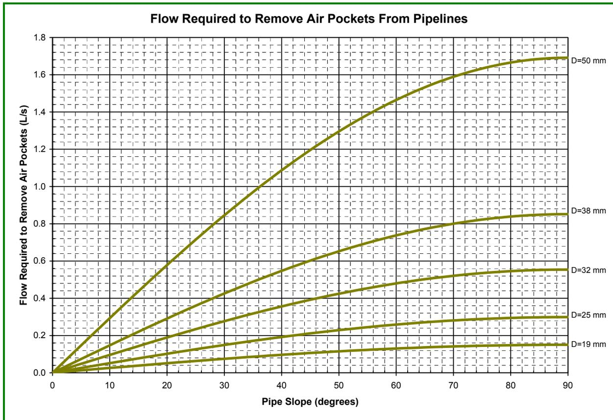
Graphic Text to Translate: Flow Required to Remove Air Pockets from Pipelines; Flow Required to Remove Air Pockets (L/s); Pipe Slope (degrees); D=19mm
