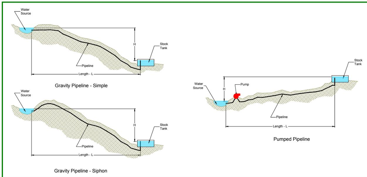
*Graphic Text to Translate: Water Source; Pipeline; Stock Tank; Length – L; H (height); Gravity Pipeline – Simple; Gravity Pipeline – Syphon; Pumped Pipeline; pump*
