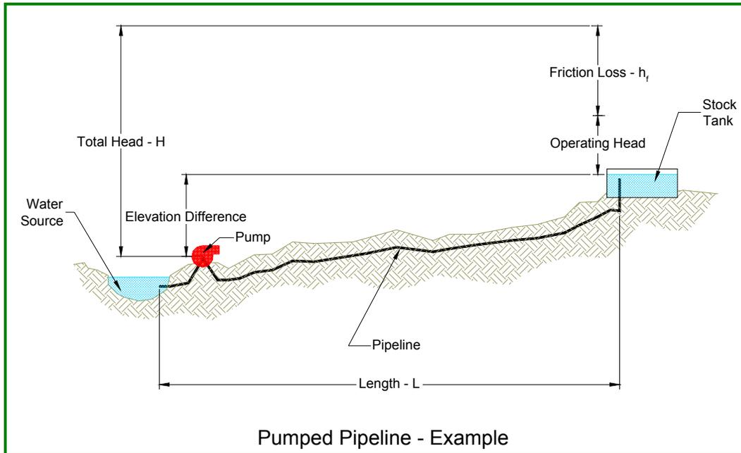
*Graphic Text to Translate: Pumped Pipeline – Example; Total Head – H; Water Source; Elevation Difference; Pump; Pipeline; Friction Loss –  $h_f$ ; Operating Head; Stock Tank; Length - L*
