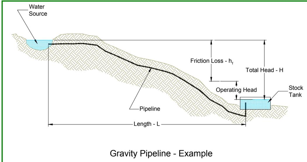
Graphic Text to Translate: Gravity Pipeline – Example; Water Source; Pipeline; Friction Loss  $h_f$ ; Operating Head; Total Head –  $H$ ; Stock Tank; Length -  $L$
